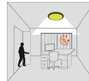
With movement and insufficient ambient lux level, the light is triggered on by the detector.
